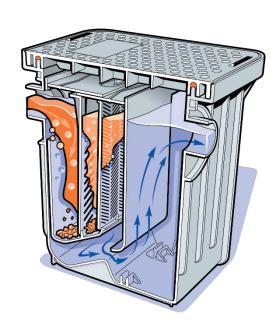
The Endura Solids interceptor should be cleaned and/or checked weekly as solids left in the tank for more than 5 – 7 days will change the pH of the interceptor.
