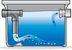
The Endura Sediment Trap can be used to separate by gravity fine material such as plaster, clay, sand, coffee grinds and general debris.
